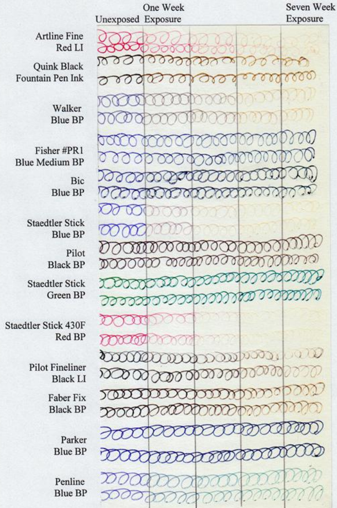
Figure 1: Effect of exposure to window filtered sunlight on various inks for periods of 0, 1, 3, 5 and 7 weeks.
